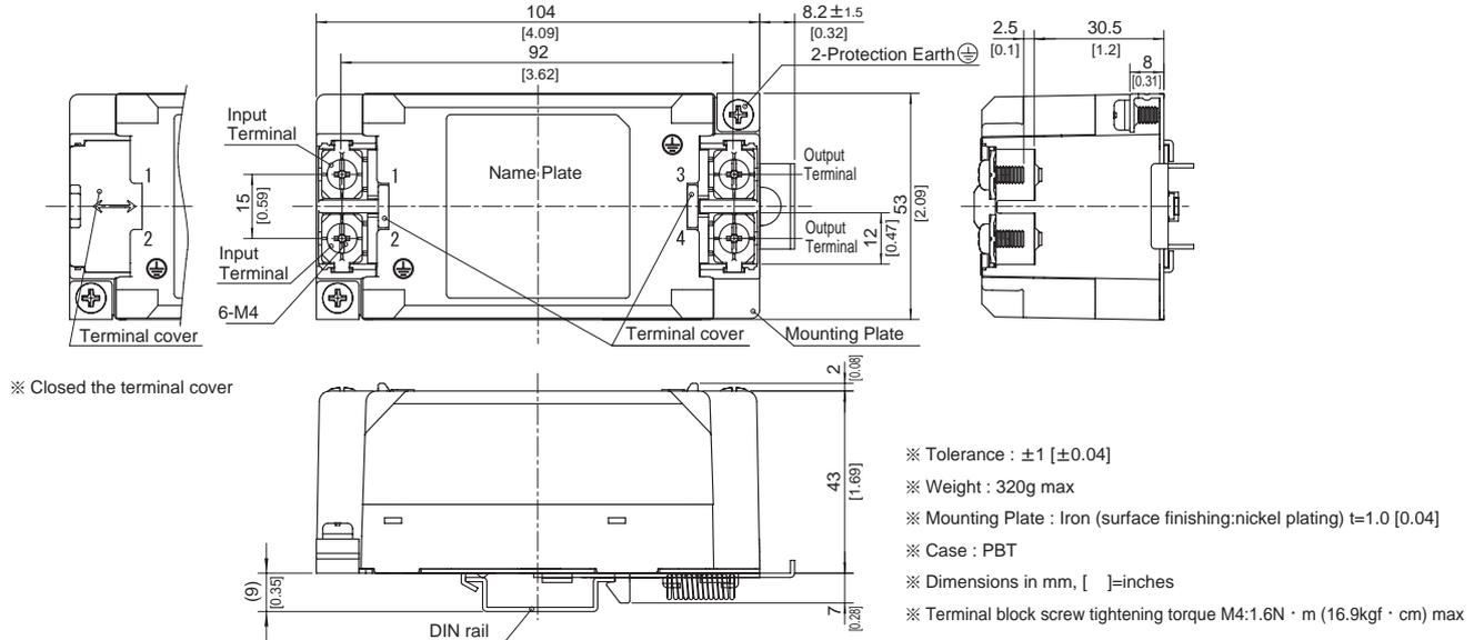
■ Note when installing the EMI/EMC Filter on a DIN rail.
