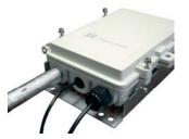
4) To better enable waterproof operation it is recommended that installers use Teflon tape to cover threads before installation. Users may also wish to use silicon sealant to further protect from ingress of liquid.
